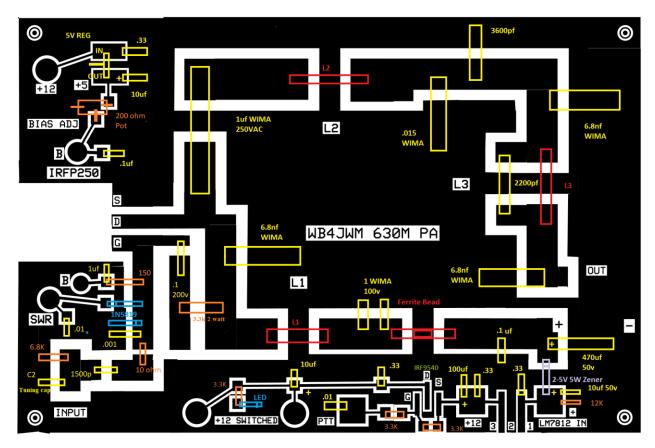
The board is populated with all the components needed for the Linear amplifier. The bias circuit is not needed with class E Amplifiers. Not shown but a jumper is needed from tab B to B for the linear amplifier.
