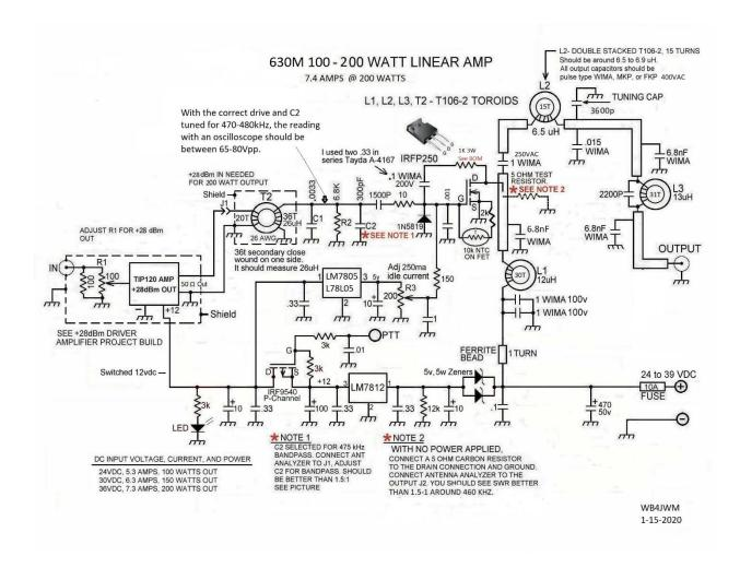
LINEAR AMPLIFIER USING THE CIRCUIT CONFIGURATION ON THE PCB. If not building linear just don't add the LM7805 bias circuit and connect the 150 ohm resistor from Gate to ground.
